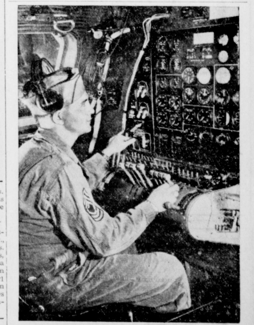
FLIGHT ENGINEER is seated before dial array on B-29 Superfortress in first photo released by War Department. Addition of engineer leaves pilot and co-pilot free to concentrate on flying technique and combat strategy. Engineer handles basic mechanical operations.
