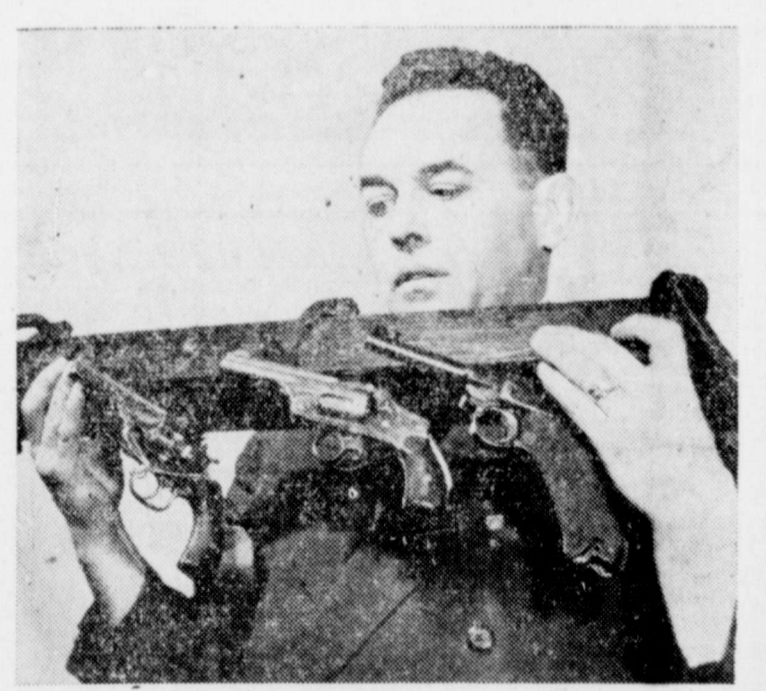
CRIME DETECTOR —New type electro-magnet used to recover revolvers and other criminal weapons from lake or river bed will lift nearly 175 pounds. Director Charles Wilson of Chicago Police Crime Detection Laboratory displays device made of alloy compound of aluminum, nickel and cobalt. Guns cling to magnet.
