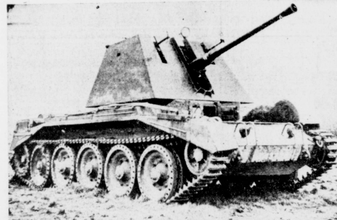
SELF-PROPELLED CRUSADER —This immense anti-aircraft tank with tracks making it adaptable on any terrain protects British convoys in Europe from low-flying aircraft. Self-propelled tank is called Crusader and has gun turret which revolves just as anti-aircraft installations do.
