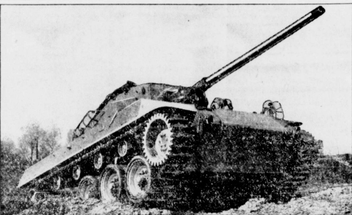
FIRST PICTURES of the M-18, a high speed, heavy fire-power tank destroyer have been released by military authorities following the battle baptism of this new super weapon. Capable of speeds of 55 miles an hour, it mounts a high velocity 76 MM cannon which can knock out enemy tanks point blank at several thousand yards. Designed and manufactured by the Buick Motor Division in cooperation with the Army Ordnance, it has been in secret production for more than a year and is now in effective action against tough enemy resistance points in the European and Pacific battle areas. It's called a "Hellcat".
