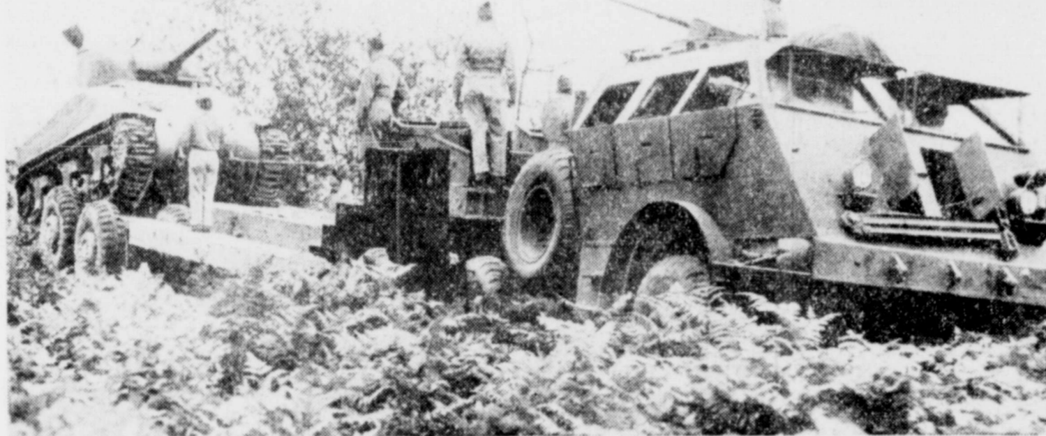
TANKS RIDE TO BATTLE—Army tanks now enter battle with full fuel containers and with cool motors, through use of new device called tank recovery vehicles. Vehicles weighing more than 40 tons carry tanks or other armored pieces into battle or withdraw disabled ones for repairs. Each vehicle is armed to protect itself from enemy ground and air attack and can operate for four days entirely on its own.
