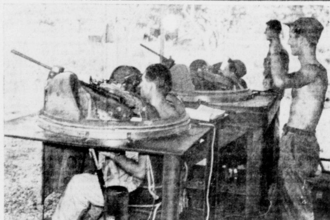
TURRETS FOR PRACTICE—Gun turrets taken from wrecked planes and equipped with shotguns serve as ideal practice weapons for students at a bomber gunnery school in New Guinea. Instructor at right signals for clay pigeon release.
