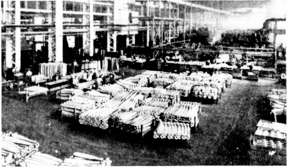
The blades that put the power into the wings of Victory for the United Nations constitute an important war production project for the Chevrolet Motor Division of General Motors. Shown above is a scene in one of the four forging hammers in this vast unit of "the arsenal of great aluminum forge plants in the Chevrolet manufacturing system, plants whose combined output of aluminum aircraft forgings is attaining record proportions. Propeller blades are forged from aluminum bar stock on giant forging hammers in this vast unit of "the arsenal of democracy."
