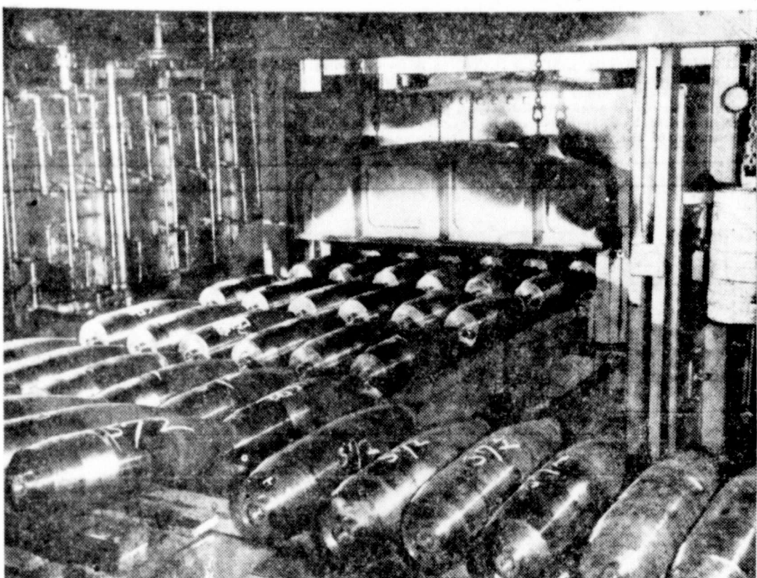
INTO THE OVEN—Marching six abreast, a covey of rough-turned 155 mm. shells marches into oven at Willys-Overland plant, Toledo, for heat treatment.
