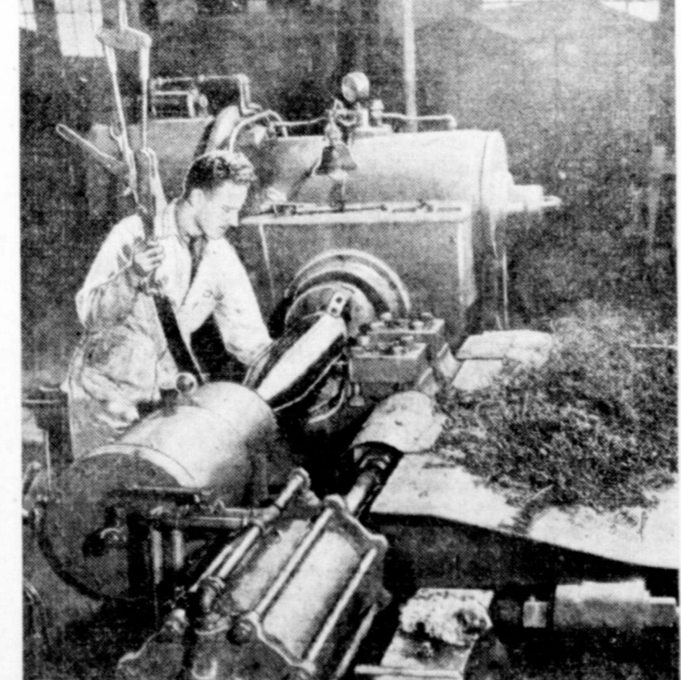
Shaving a 7.2-inch howitzer shell on a giant lathe. The Dominion's ammunition factories make 18 types of shells in 14 different calibres. They employ 50,000.
