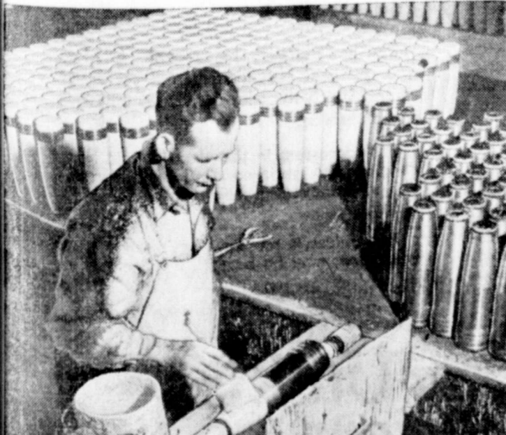
Applying paint on 3.7-inch anti-aircraft shells, one of many produced under the vast shell and bomb program of the Department of Munitions and Supply.
