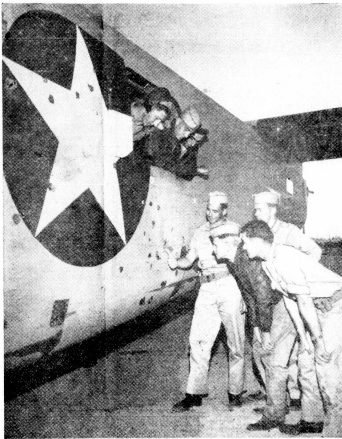
TWO HUNDRED SOUVENIRS—Despite two severed control cables, 200 holes in its fuselage and a left aileron almost torn away, this American B-24 Consolidated bomber got back safely to its base from long bombing flight in Libya. Crew members survey the scars of battle. (O.W.I. Photo)
