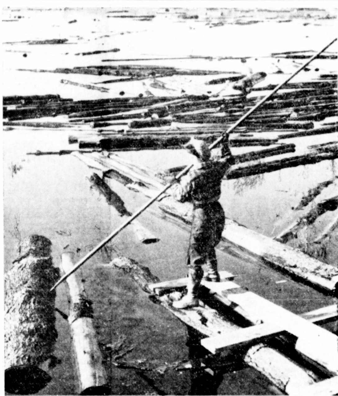
LUMBER MISS—Eighteen-year-old Norma Webber, one of eight women employed at New England Timber Salvage Corp., Concord, N. H., uses a "pick pole" to bring in a log, at sawmill to which logs are floated downstream from timber camps. Girls are filling gaps in labor ranks caused by inductions.
