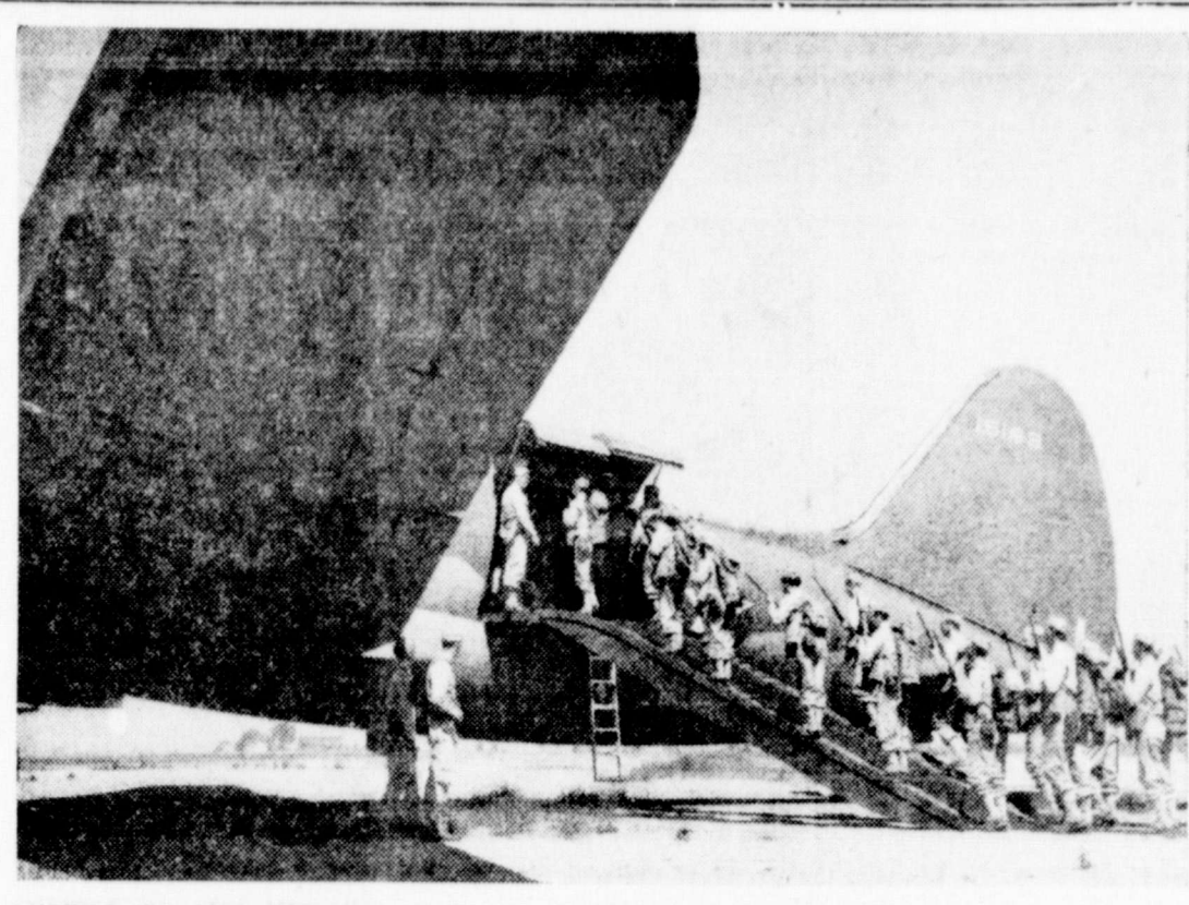
ANSWER TO SUB MENACE —Fully equipped U. S. infantrymen enter spacious cabin of a new giant Curtiss-Commando military transport, world's largest twin-engine airplane, during tests which proved plane's ability to transport scores of troops and their equipment, light artillery and jeeps.
