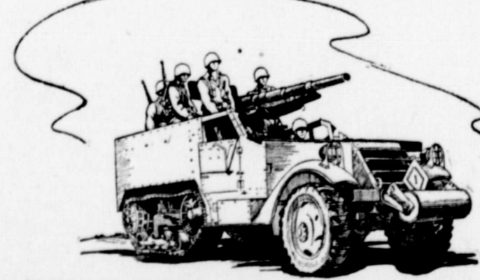
DESTROYER ON LAND—A heavy, rapid-fire cannon mounted on a half-track armored car, that's the self-propelled artillery, the answer to the Armored Force's need to thrust heavy artillery firepower directly into the core of its lightning attacks.
