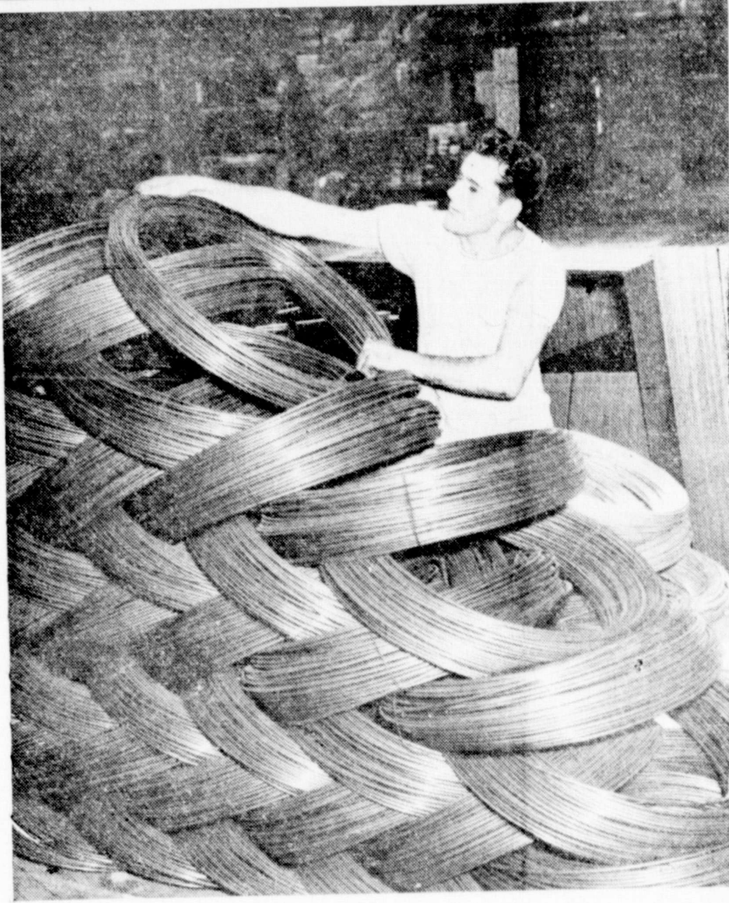
WIRE CONVERTED TO SHRAPNEL—At one of the many small household appliance plants on the West Coast that have been converted to war manufacture, a workman stacks coils of wire that are to be cut up for shrapnel. Plant formerly turned out window screens and weather strips.
