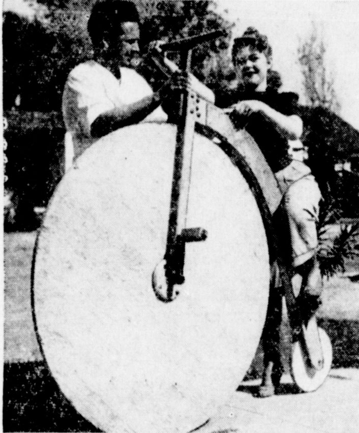
FOR RIDING HIGH—To beat rubber shortage Dr. Don Truitt, left, of Long Beach, Calif., devised this plywood high-wheeler. Lorraine Foreman gets the first ride.
