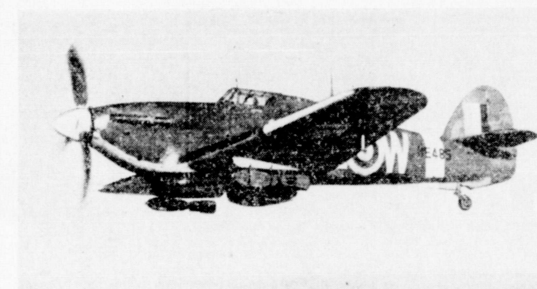
HURRICANE AND BOMBS.—To increase the power of the RAF in low level attacks, Hawker Hurricanes are now equipped to carry bombs fitted with delayed action fuses to enable the aircraft to get clear before the explosion. Bomb racks and load can be clearly seen in the above photo.
