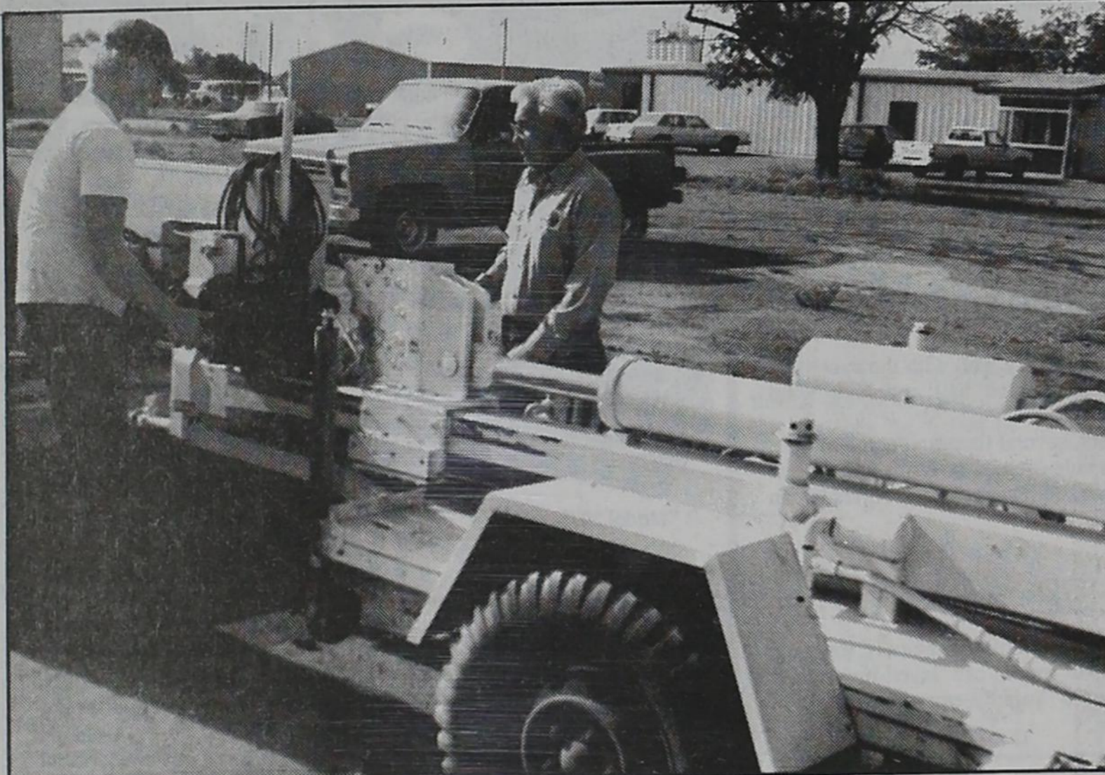
THE SHREDDER—Operating the city's new tire-shredding machine are (from left) city employees Jeff Howell and Ralph Salinas. The machine was constructed by city employees James Killough and Salinas at an estimated cost of $1,600, in comparison with a new machine that could cost as much as
