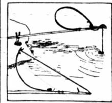
spring, one end of which is securely fastened to the pole at some distance from the end. The free end carries the fishing line and means for engaging a trigger, which is designed to be sprung by any movement of the line. In order to make the sport still more mechanical an audible signal of some kind is provided, which announces to the fisherman that the line has been sprung should he not be watching closely at the moment.
