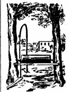
Nature, as well as necessity, mothered the invention of the lathe, the originally between two adjacent large trees near which grew a springy sapin some of the Asiatic countries.
