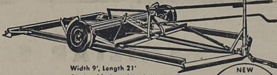
Width 9', Length 21' Cutting blade 6' 3" x 16" Weight 1200 lbs., 2 Plow Tractor
