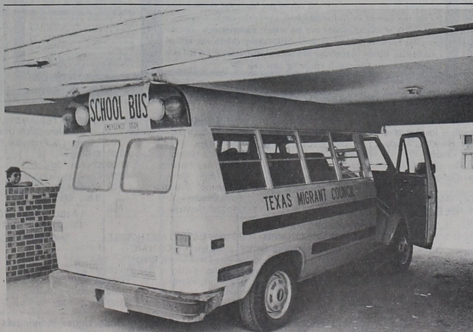
WOOPS! —The canopy at Al's Colonial Restaurant has a clearance of 7'3". But the extended roof of the Migrant Head Start school bus is 7'8" high. The driver found it out the hard way last Thursday
