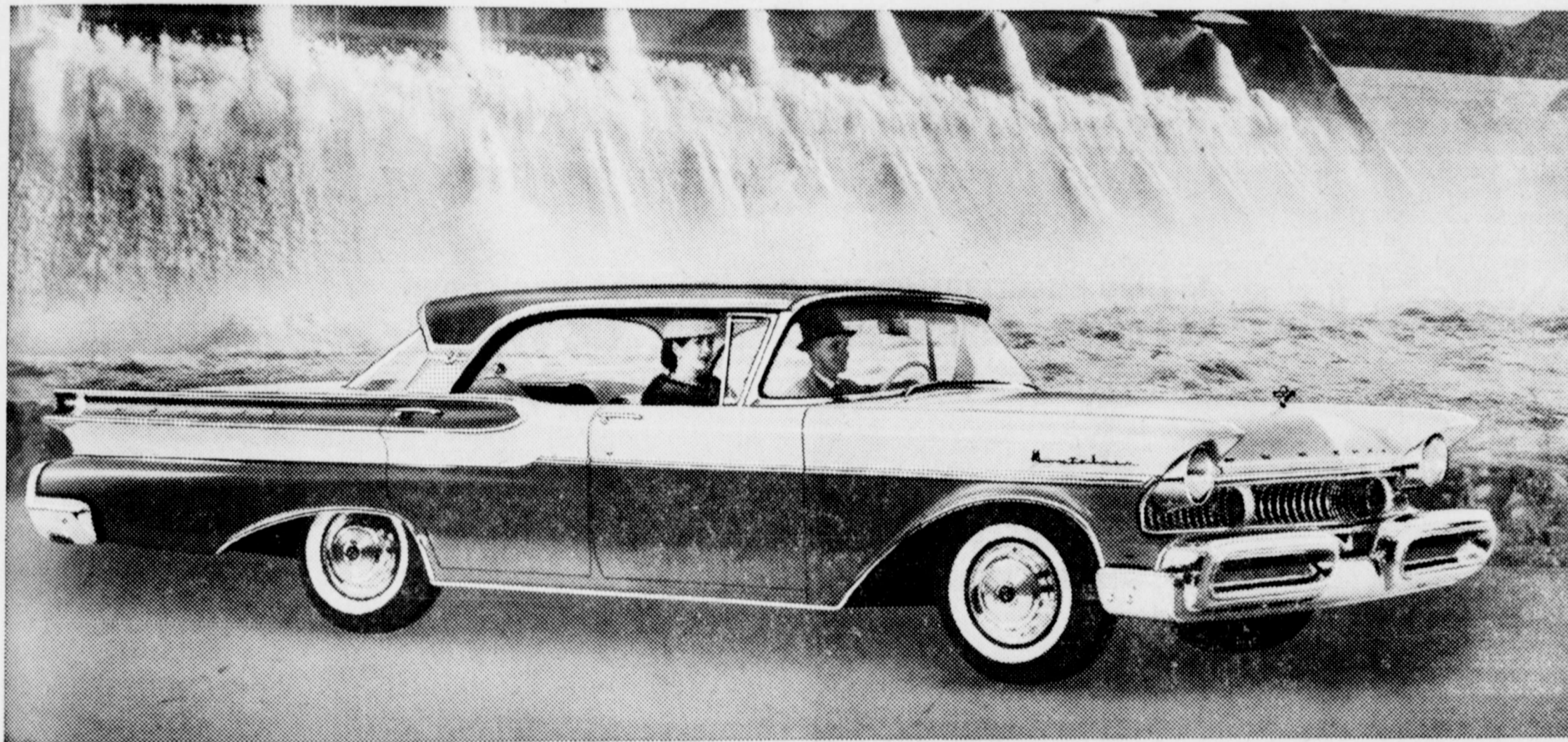
BIGGEST SIZE INCREASE IN THE INDUSTRY —Mercury is now over 17½ feet long, more than 6½ feet wide. Wheelbase is a big 122 inches. Inside there are inches more headroom, leg room—as much shoulder room, for example, as in many of the most expensive cars.
