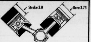
Here's the measure of a truly modern V8 engine -Chevrolet's advanced oversquare design. It means less friction . . .
