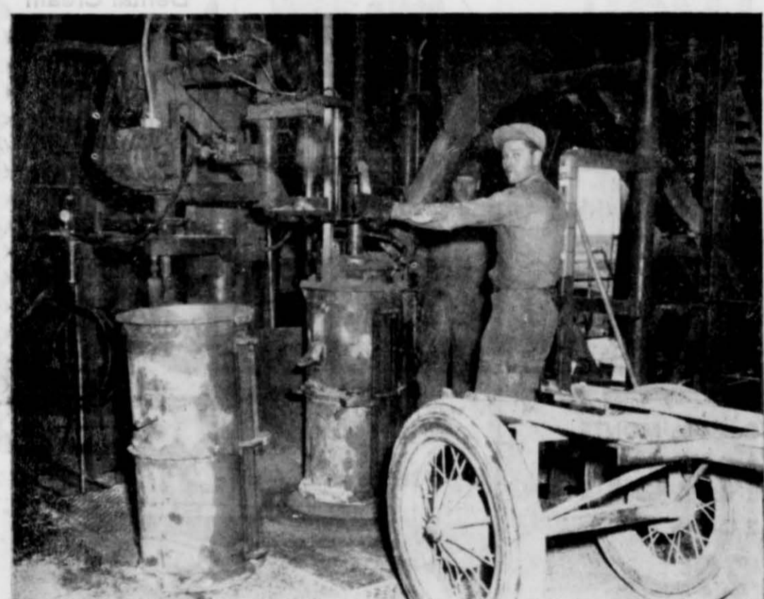
The concrete pipe-making machine in operation is a fascinating sight. Semi-automatic in operation, it can be operated by one man while several others take out the lengths of pipe. A conveyor belt carries a mixture of gravel and cement to the revolving mold (under operator's left hand) where it is tamped while poured at about 800 strokes per minute then taken out. Much machinery is involved in this one piece of equipment to turn out our current production of 1,200 to 1,300 feet of pipe a day, or 400 3-foot sections.
