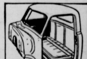
Battleship-construction double-walled cabs
