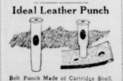
By using the size rifle cartridge shell desired, leather punches may be made. Holes cut in the side of the shell enable the emptying of leather without trouble.
