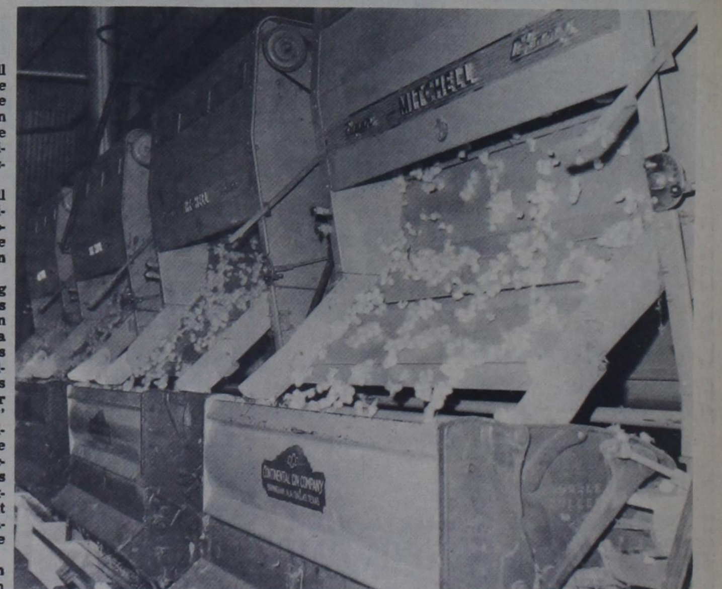
A FEW BALES of cotton are being ginned in the county as shown by these gin stands at Dimmitt Gin. The major portion of the white money crop is still in the farmer's field awaiting a killing frost. The unusual warm November days are delaying the cotton strippers. —Staff Photo
