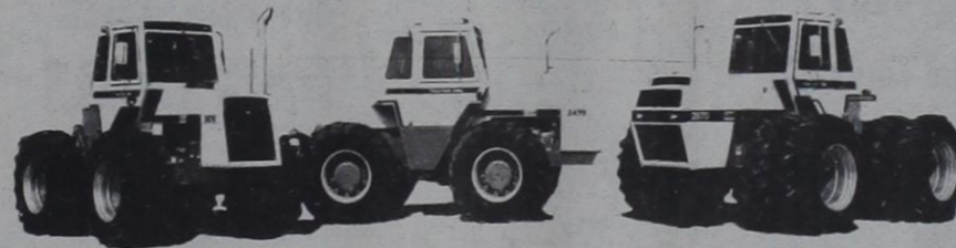
2670 *256 engine hp 221 PTO HP 2470 *213 engine hp 176 PTO HP 2870 *300 engine hp 252 PTO HP *Manufacturer's rating, all others official test.
