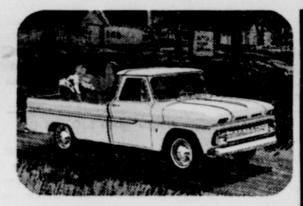
FLEETSIDE. Based on sales, the best liked pickup in the world. Outstanding feature is its large body extending clear out over the wheels. Two body sizes. Two wheelbases. Best riding truck, by far, with coil springs all around and independent front suspension. Cab and body have doublewall construction. Chevrolet Fleetsidebest for all-around use.
