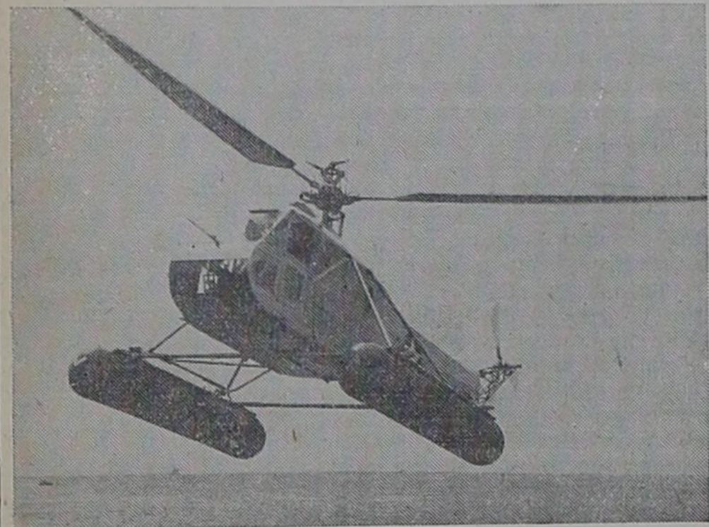
This Sikorsky type of helicopter, which will be built in quantity for the Army Air Forces by Nash-Kelvinator Corporation, peacetime manufacturer of automobiles and refrigerators, can alight on land, water, snow, thin ice, a rooftop or a parking lot. The craft can hover motionless in mid-air; descend and ascend vertically without forward motion and fly backward, sideways or forward with equal facility.
