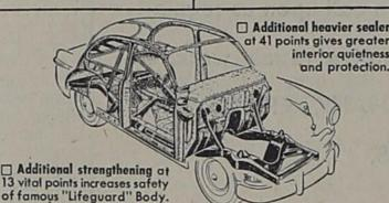
☐ Box-type frame rails have steel of increased thickness
