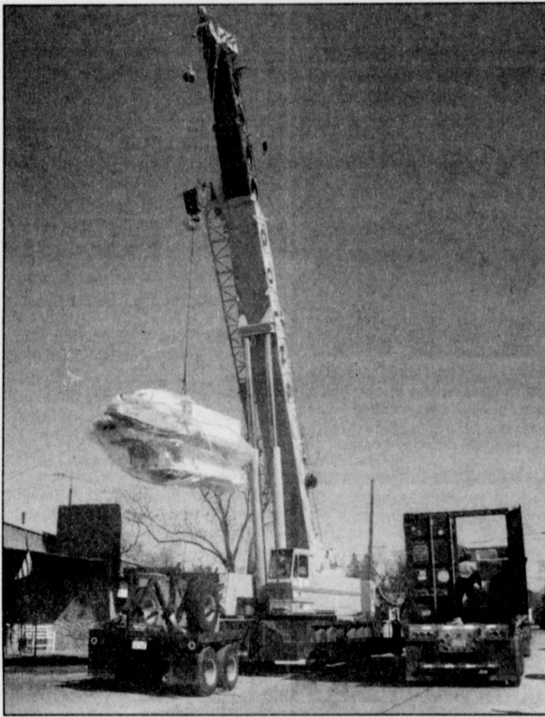
A NEW PUNCH PRESS from Trumpf, Inc. of Germany is unloaded and moved into a building at Contico (John's International). Employees Fred Fortson and Larry Nitsch spent two weeks in Connecticut for training in operation and programming of the press which weighs 50,000 lbs. and cost approximately $473,000. (photo by Jean Boles)
