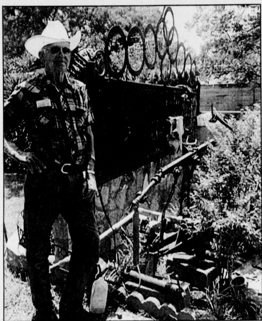
DEWEY CHESTNUT, 81, stands beside his unique water pump he built using an old window weight, lawn mower parts, evaporative air conditioner parts, a grease gun, professional meat grinder, a bicycle fork, PVC pipe, and concrete rebar. The slow but steady contraption pumps 3-4 gallons of water per hour from his backyard well.
