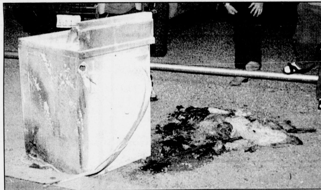
BURNED WASHER AND RAGS were brought outside the gymnasium following a small fire last Thursday evening. According to Winters Volunteer Fire Dept. chief Jack Davis, Jr., some greasy rags had been washed and dried then placed in a plastic container. The heat in the rags was apparently sufficient to cause the rags to ignite, starting a fire in the washroom of the gymnasium which sustained some smoke damage. See related story.
