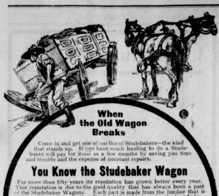
This reputation is due to the good quality that has always been a part of the Studebaker Wagons. Each part is made from the lumber that is best fitted for that part. New England black birch makes the best hubs—the Studebaker hubs are made of it. Butt cut, second growth black hickory is the best for axles—Studebaker axles are made of it. Selected white oak is best for spokes and running gears—that is what is used in the Studebaker Wagon. The Studebaker Wagon
