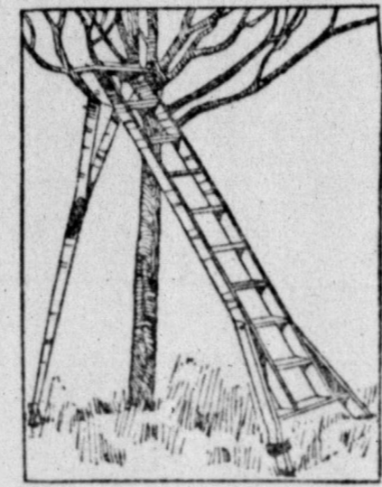
Three-Legged Stepladder—Stands Firm on Uneven Ground—Substantial and Easily Handled by One Man.
