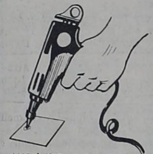
USE A HOT-MELT GLUE GUN TO MOUNT THE PHOTOS. THE GLUE IN A NEW GUN MADE BY WELLER SETS IN 20 SECONDS, WHILE THE HANDY STAND PACKAGED WITH EACH GUN ALLOWS THE USE OF BOTH HANDS FOR POSITIONING THE PHOTOS.
