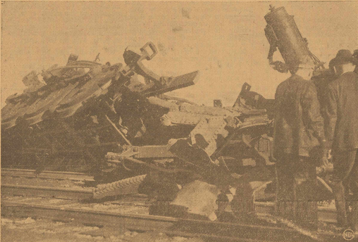
Three men were killed, the boiler was hurled 300 feet, rails were torn up and a great hole dug in the road bed when a railroad locomotive exploded between Elgin and Almore, Ill. The above picture shows the tangle of twisted and broken metal that was left when the locomotive of the Chicago, Milwaukee, St. Paul & Pacific railroad let go with a roar. A fireman, an engineer and a brakeman died in the wreckage.
