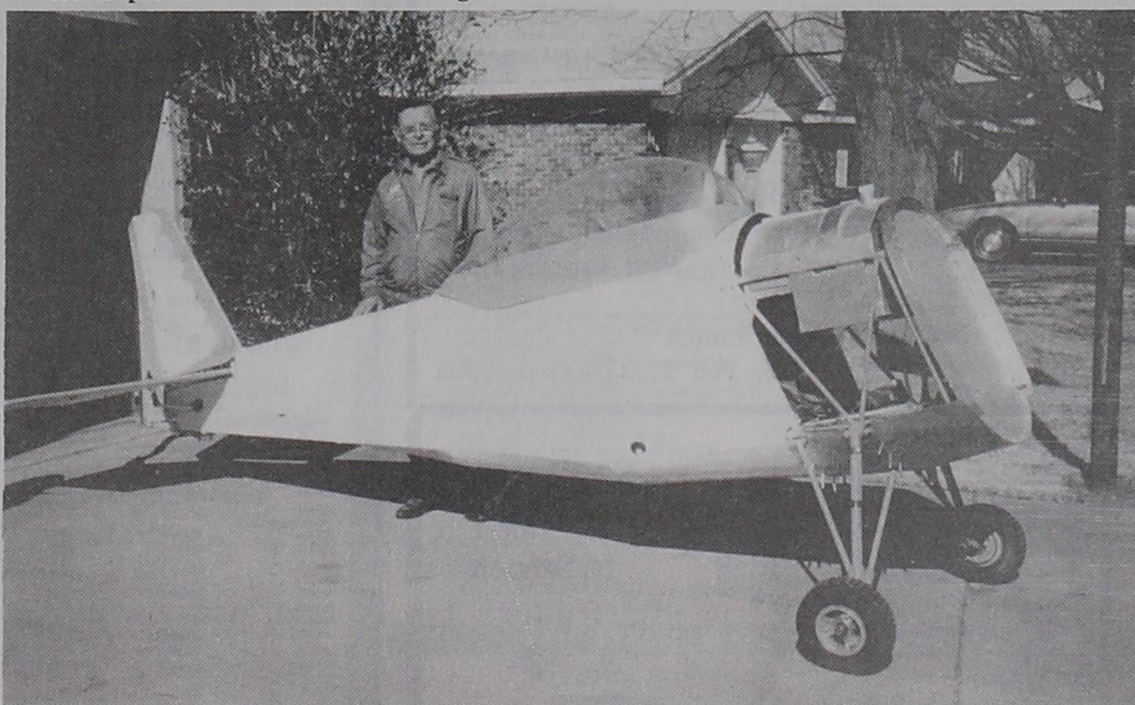
SOMEDAY IT'LL FLY... Lew Longmire stands beside the airplane he is building in his garage on Columbia Street in Friona. The 15-foot fuselage will be outfitted with 19-foot wings and will fly 130 miles per hour. ron carr photo
