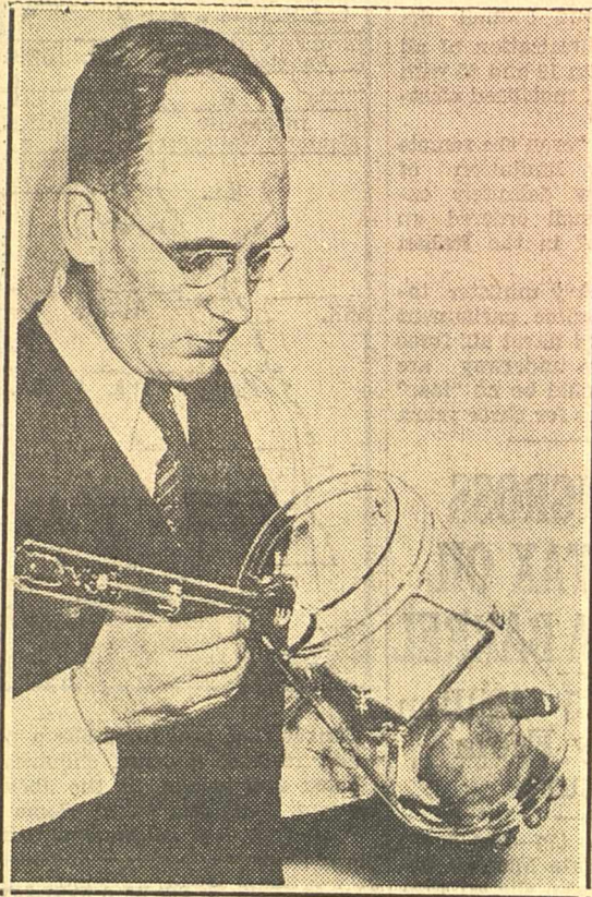
Development of the electric eye, such as P. J. Konkle inspects above, now makes possible pictures of 441 lines, about 25 per cent more than ever before. The more lines to the picture, the clearer it is, the more detail it shows.
