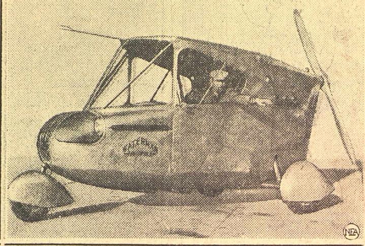
Above it's an airplane and below it's an auto. And that's about the exact status of this "Arrowbile," the invention of Waldo Waterman, Santa Monica (Calif.) plane builder. Above the ground it flies. On the ground at the airport, Waterman merely parks the wings and chugs away. The craft makes 125 miles an hour in the air; 55 on the ground.
