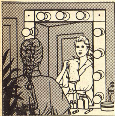
Dressing, grooming and applying makeup require balanced, bright light. Light from sides and above to achieve the best effect.
