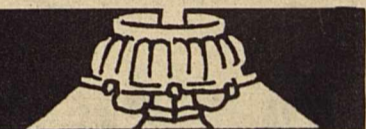
The small metal hoop on a lamp that supports the shade is called a harp.
