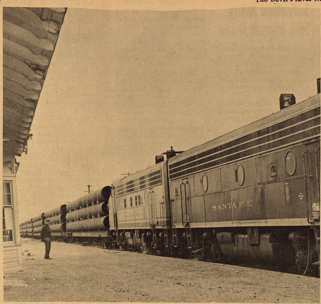
THE FIRST LOAD OF THESE HUGE 36-inch pipe 90 feet long. Each trailer carries nine of the big pipe that will be used in the construction of a pipeline for Intratek Gas Company. Presently the 28-cars are being unloaded and the pipe moved by brought in by rail. These flat cars are normally used to carry truck-trailers, and they are normal-
