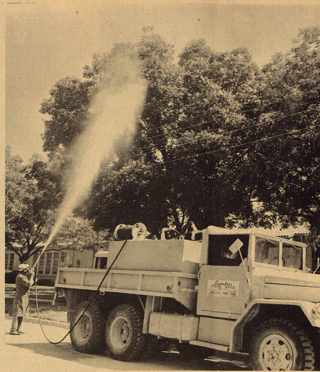
CAPABLE OF REACHING THE TOP of the tallest pecan trees is the boast Alan Saunders makes of this specially equipped sprayer truck. The 2 1/2 ton truck was selected for use in both town and country, and has 5 forward speeds and 4 wheel drive. The 1,100 gallon tank has 150 feet of hose and the pump operates on a spraying pressure of 675 pounds, although it can go as high as 800 pounds.
