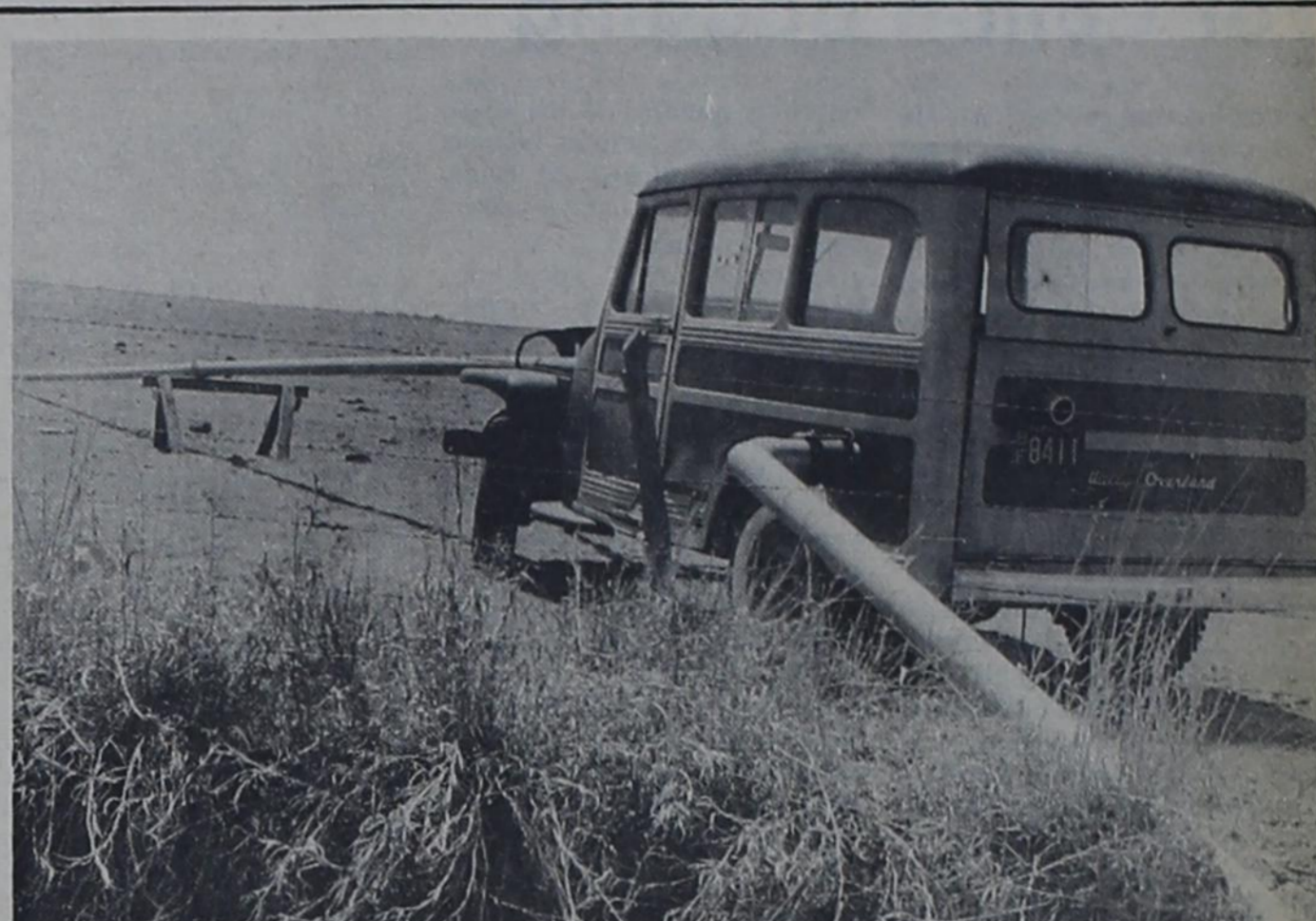
UNUSUAL TAILWATER PUMP on the Leon Hart farm north of Friona is formed by this jeep, which has a motor in the back for pumping water, and the pipeline running through the back of the jeep and out through the headlight. It also is handy in that it is mobil.
