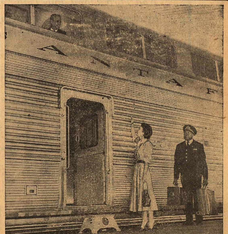
HI, LEVEL!—Pretty miss waves a greeting to fellow passenger as she prepares to board one of Santa Fe Railway's new experimental Hi-Level chair cars, to be used in test runs on El Capitan, The Chief and the San Francisco Chief. Upper deck of cars is devoted entirely to chairs for 67 passengers, with lower deck for baggage storage, rest rooms and service equipment.
