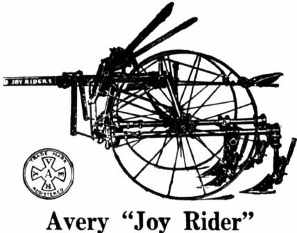
Side levers after being set changed without stopping to give the desired depth of the team, and wheels can be cultivation need not be set as close together as 40 touched, making it easy inches or as far apart as 48
