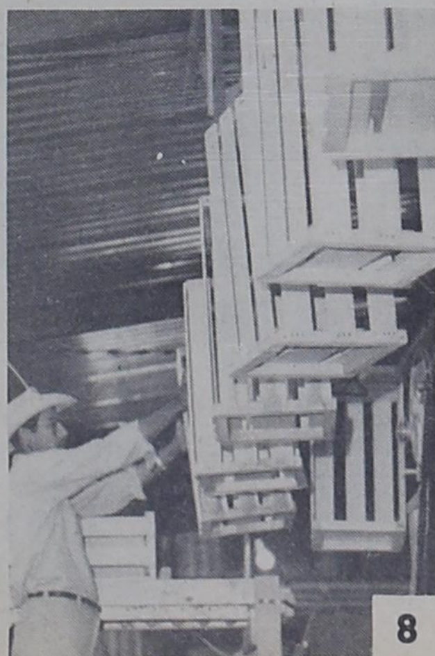
A man must continually replace empty crates on a winding conveyor which carries them to the speedy packers.
