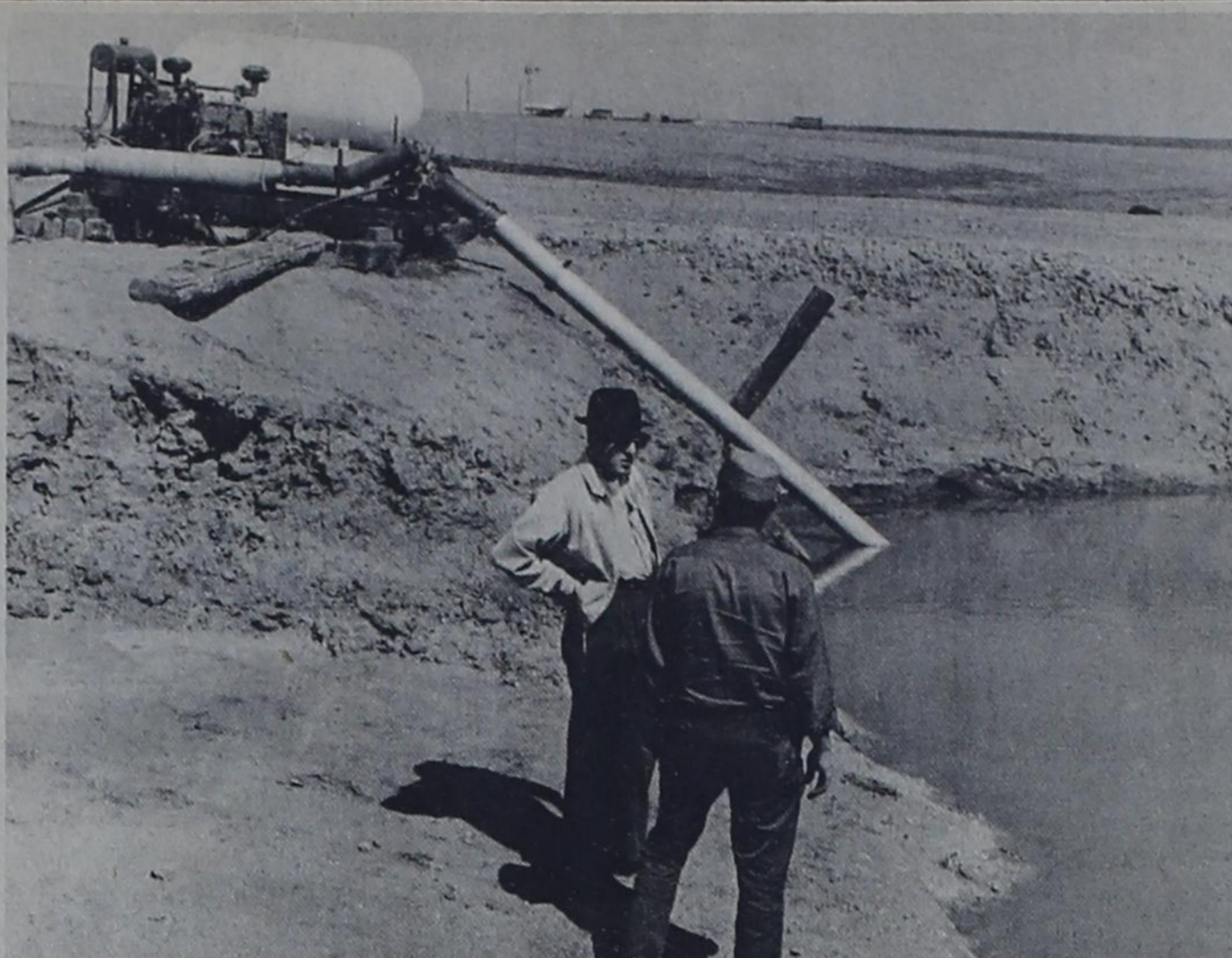
ONE OF THE COUNTY'S many lake pumps in the area which makes use of tailwater is this one, located on the Gilbert Wenner farm south of Friona. Wenner's pump has been gauged at 72,000 gallons per hour. Allan White and Wayne Wyatt of the High Plains Underground Water Conservation District are seen in the foreground.
