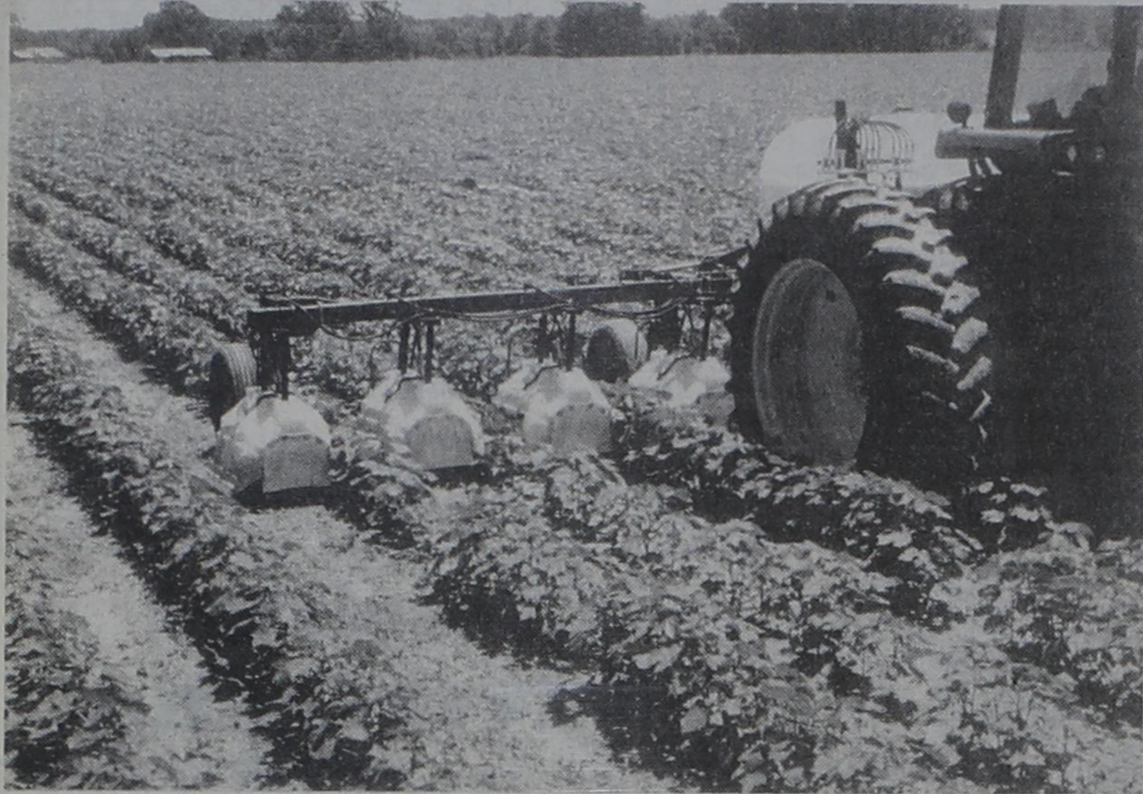
HOODED SPRAYERS..... Growers opting to use hooded sprayer equipment are finding many advantages to the reduced-tillage system, especially with the wet weather. Hooded sprayers are quickly becoming a sound alternative to cultivation for growers throughout the South.
